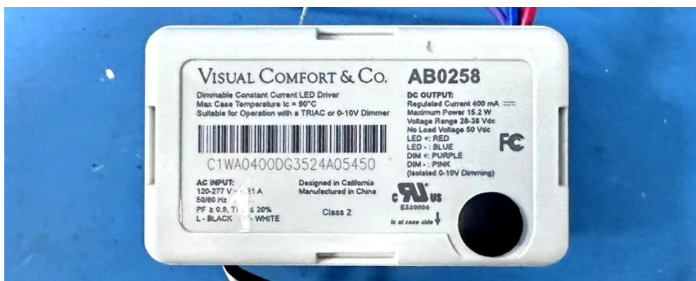
View of LED driver PTB20W-0400-38-VCC1(AB0258)
